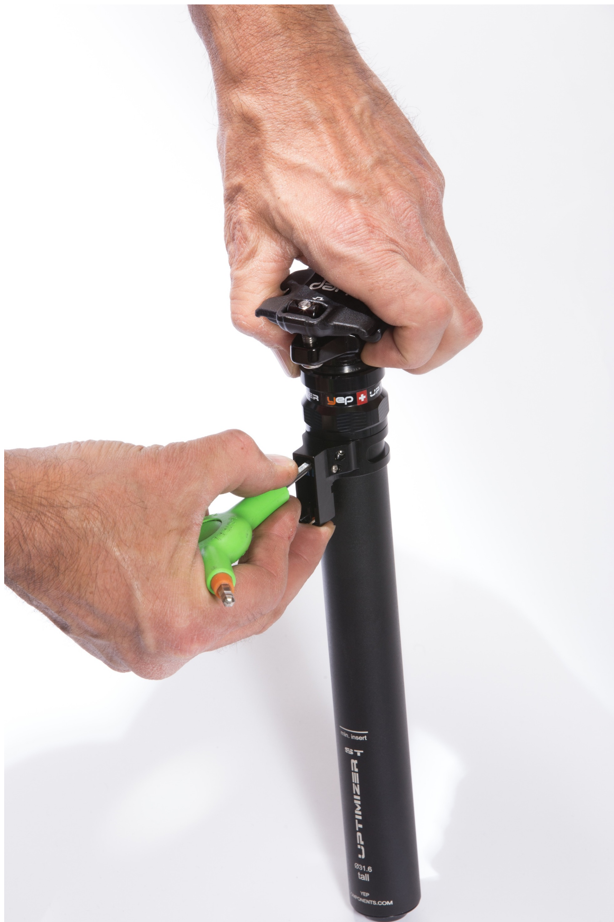
1) place the seatpost on a stable surface and use a tool to rotate the actuator rocker
