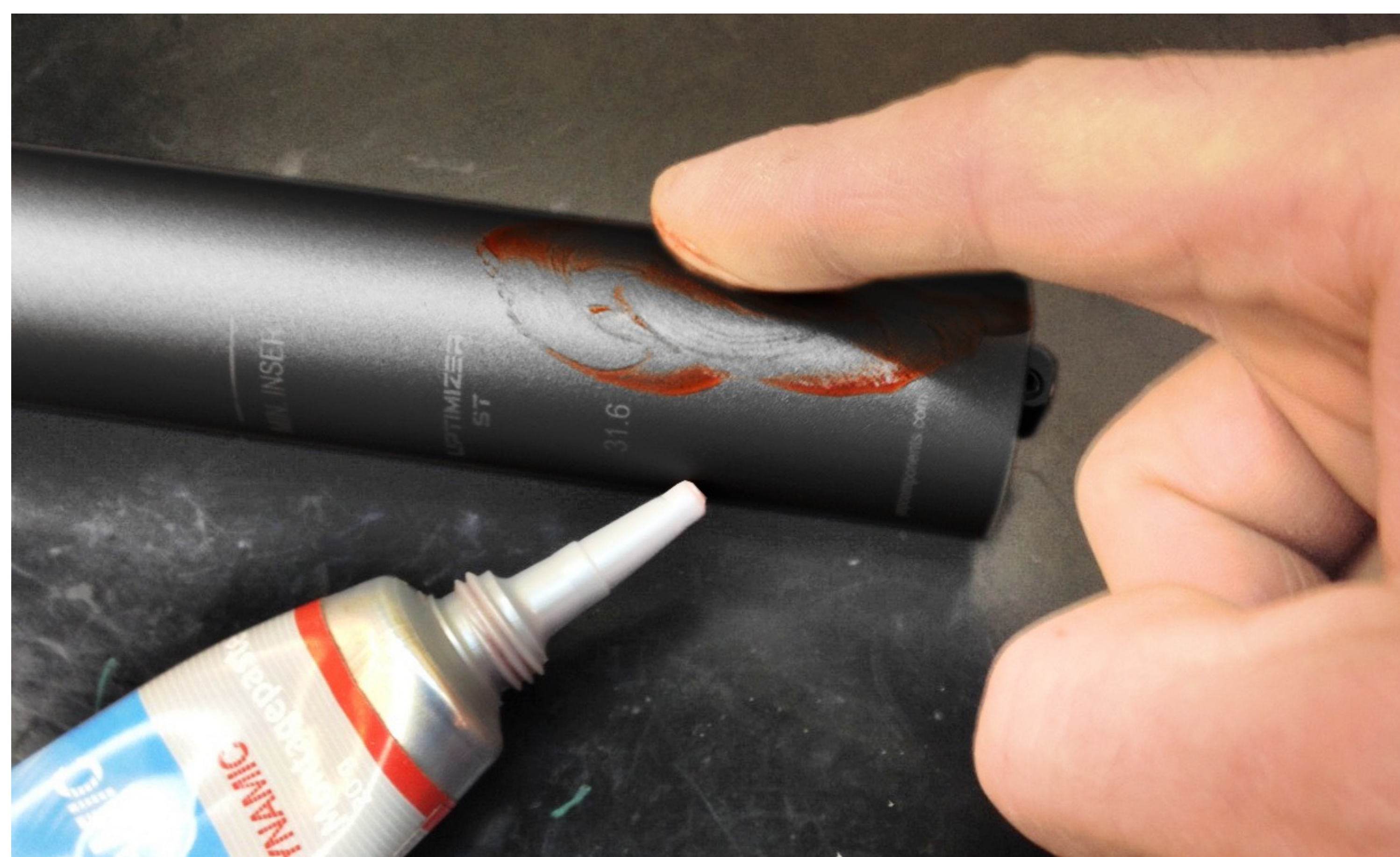
3) apply a small quantity of friction paste (do not use grease)
