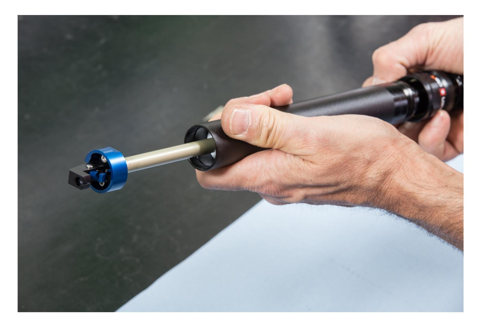
• Use internal snap-ring pliers to remove the bottom lock ring
