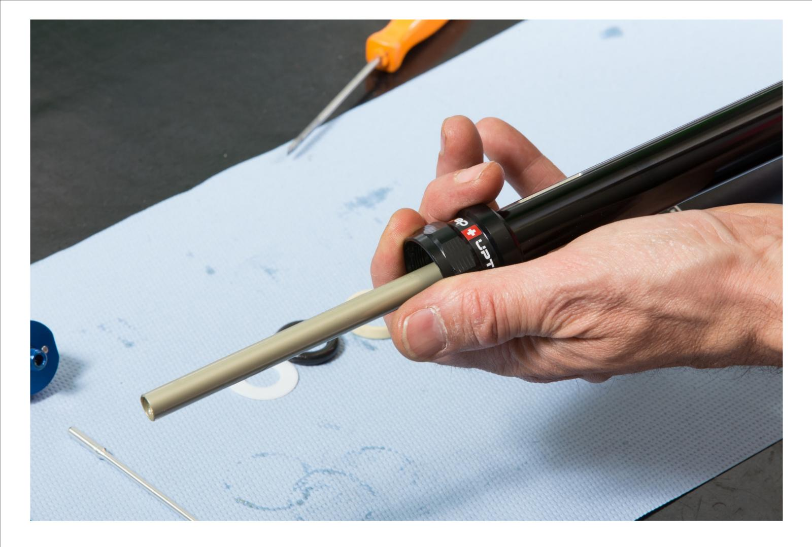
• Carefully reinstall collar, paying attention not to damage the lip of the dust ring
