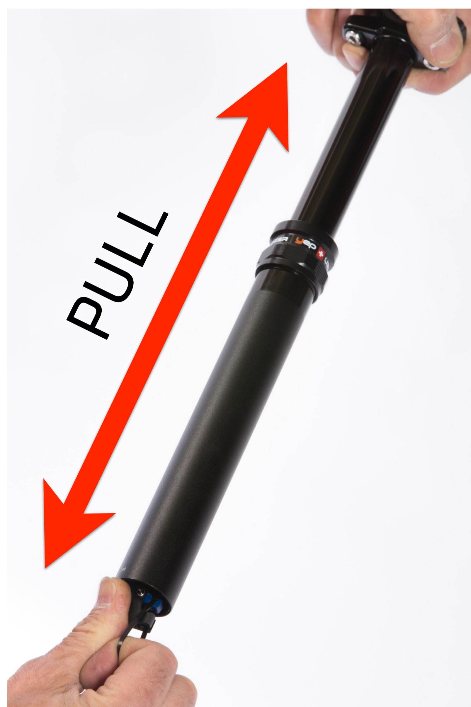
5) pull both ends to extend the seatpost
