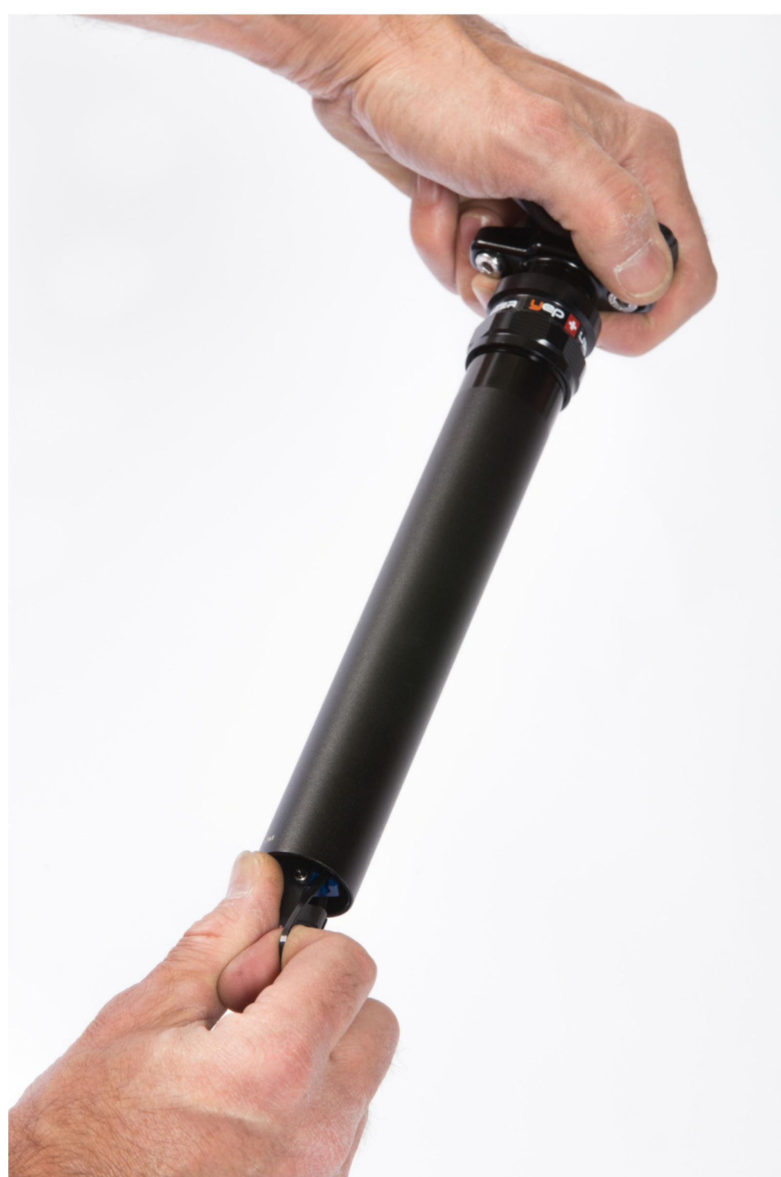
4) pull the release lever to the open position
