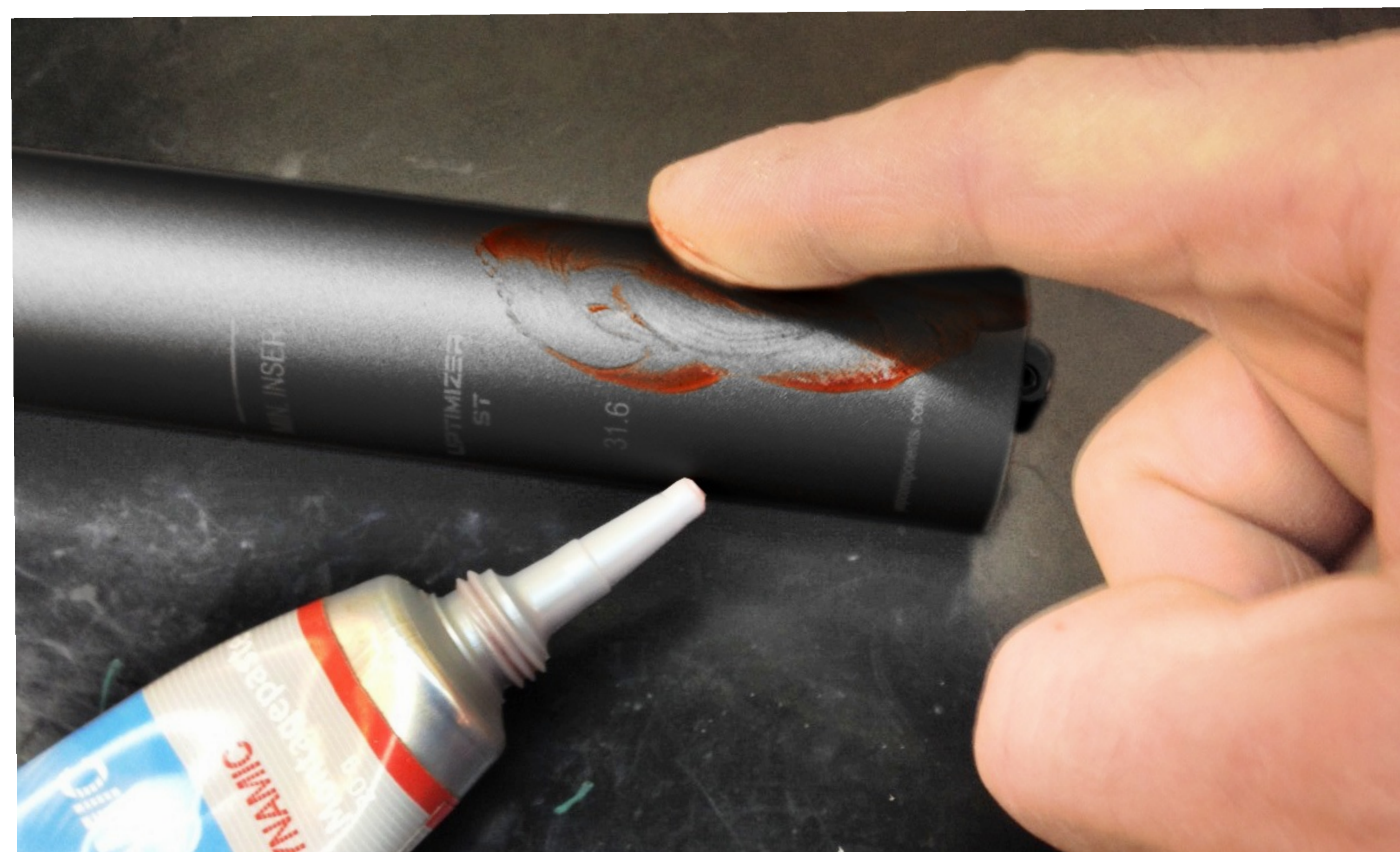
6) apply a small quantity of friction paste (do not use grease)
